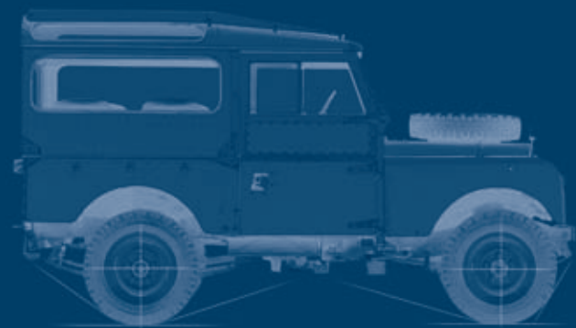
Series I Station Wagon (1954-1958) 1954 Long-wheelbase 107 inch available 1957 First diesel engine introduced.
